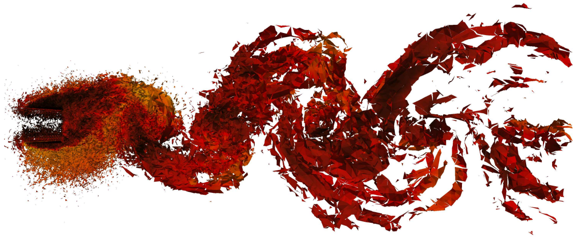
Figure 21: Isosurface of the q -criterion colored by velocity magnitude showing the wake behind the square cylinder
